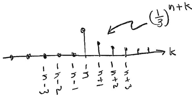
Third step: flip the graph with respect to the  $k$ -axis.
