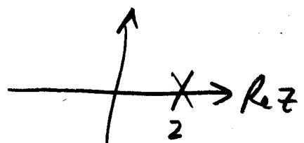
→ The causal system is unstable because the pole at  $z=2$  is outside the unit circle.
