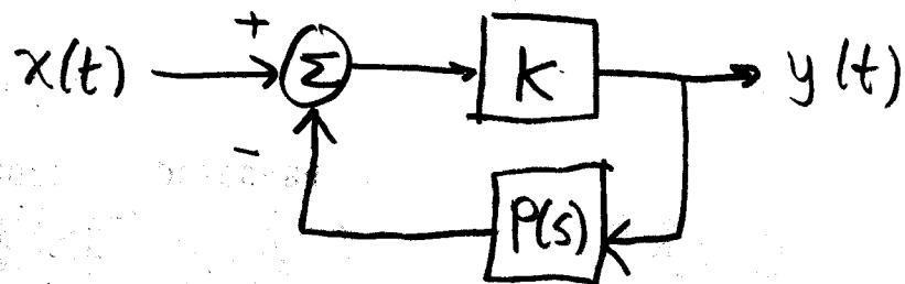
$$\begin{aligned} Q(s) &= \frac{K}{1+KP(s)} \\ &\approx \frac{K}{KP(s)} \\ &= \frac{1}{P(s)} \quad ||, 7 \end{aligned}$$
