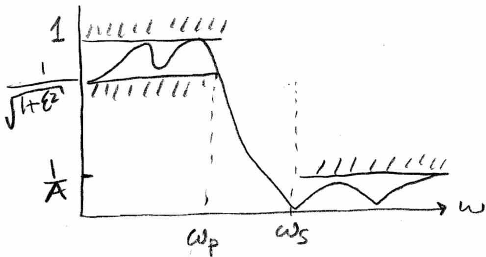
The critical frequencies may be specified in (analog) Hz or radians along w/ a sampling frequency ... in cases where the the digital filter will be used to implement an analog filter.
