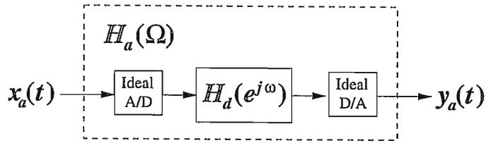
The sampling frequency of the A/D and D/A converters is  $F_T = 2 \text{ kHz}$ .
