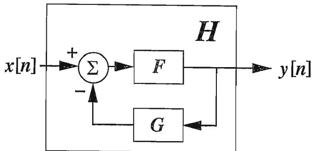
The purpose of the feedback is to stabilize the system  $F$  by moving the pole. The impulse response of LTI system  $G$  is given by  $g[n] = K\delta[n]$ , where  $K \in \mathbb{R}$  is a real constant.
