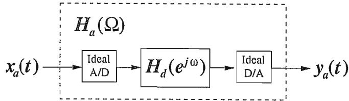
Assume that all input signals  $x_a(t)$  are band limited with  $|X_a(\Omega)| = 0 \forall |\Omega| > \pi/T$  so that aliasing does not occur.
