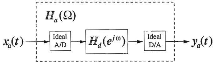
The sampling interval of the A/D and D/A converters is  $T = 1$  sec, so the sampling frequency is given by  $\Omega_T = 2\pi/T = 2\pi$  rad/sec. All input signals  $x_a(t)$  are bandlimited to  $|\Omega| < \Omega_T/2 = \pi$  rad/sec (this simply ensures that the overall structure shown in the figure will be an LTI system).
