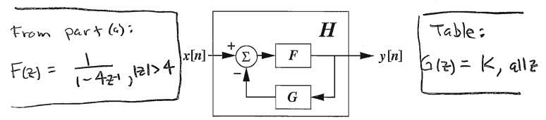
The impulse response of LTI system G is given by  $g[n] = K\delta[n]$ , where  $K \in \mathbb{R}$  is a real constant.
