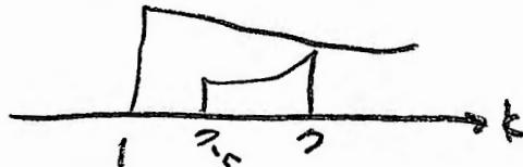
$$\begin{aligned} y[n] &= \sum_{k=n-5}^n (\frac{1}{2})^k (\frac{1}{4})^{n-k} \\ &= (\frac{1}{4})^n \sum_{k=n-5}^n (\frac{1}{2})^k (\frac{1}{4})^{-k} = (\frac{1}{4})^n \sum_{k=n-5}^n (\frac{1}{2})^k 4^k \\ &= (\frac{1}{4})^n \sum_{k=n-5}^n 2^k = (\frac{1}{4})^n \frac{2^{n-5} - 2^{n+1}}{1-2} = (\frac{1}{4})^n [2^1 2^n - \frac{1}{32} 2^n] \\ &= 2^n (\frac{1}{4})^n [2 - \frac{1}{32}] = (\frac{1}{2})^n [\frac{64 - 1}{32}] = \frac{63}{32} (\frac{1}{2})^n \end{aligned}$$
