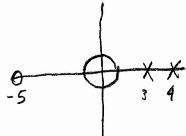
→ Use three allpass sections to trade these for a new zero & two poles that are inside the unit circle.
