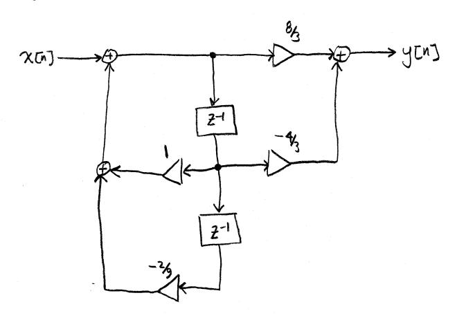
4. 25/20 pts. A digital FIR filter H has input x[n] and output y[n] related by
