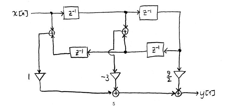
3. 25/20 pts. The causal IIR digital filter G has transfer function
