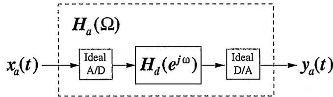
The sampling frequency of the A/D and D/A converters is  $F_T = 5$  kHz, so  $\Omega_T = 10,000\pi$  rad/sec. All input signals  $x_a(t)$  are bandlimited to  $|\Omega| < \Omega_T/2$  (this simply ensures that the overall structure shown in the figure will be an LTI system).
