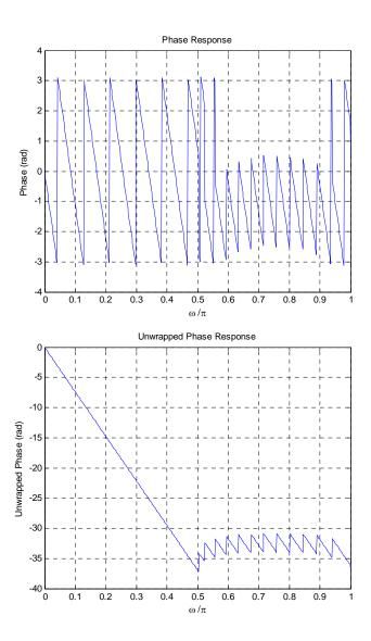
Q7.23 The MATLAB program to design and plot the gain and phase responses of a linear-phase FIR filter using firl and kaiser is shown below. The filter order N is estimated using Eq. (7.37) and the parameter  $\beta$  is computed using Eq. (7.36). The output data are the filter coefficients.
