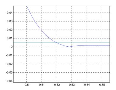
From the gain plot we observe that the filter as designed  $\underline{DOES\ NOT}$  meet the specifications. AS SHOWN in the two detail plots above, with N=46, neither the passband spec at wp = 0.4 (normalized frequency) nor the stopband spec at ws = 0.5 (normalized frequency) are met. So this design DOES NOT meet the spec.
