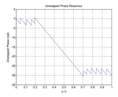
Q7.27 Using the MATLAB program developed in Question Q7.26 the linear-phase FIR bandpass filter for the specifications of Question Q7.27 is designed.
