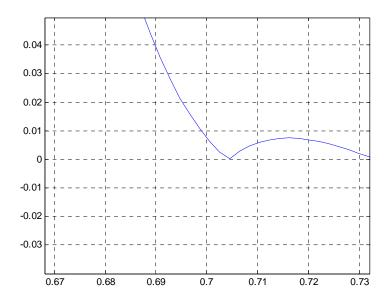
From the gain response plot we observe that the filter as designed  $\underline{DOES}$  meet the specifications.
