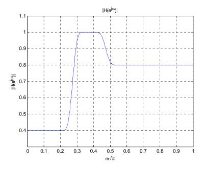
From the magnitude response plot we observe that the filter as designed <u>DOES NOT</u> meet the specifications.
