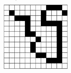
(a) 10 pts. Let the upper left pixel have coordinates (row,col) = (0,0) and consider that the LOGIC\_ONE pixel located at (1,1) is the initial pixel. Give a chain code for the contour.
