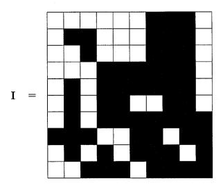
Form a new binary image  $\mathbf{J} = \text{OPEN}(\mathbf{I}, \mathbf{B})$  by applying a binary morphological OPEN filter with structuring element  $\mathbf{B} = \text{CROSS}(5)$ . Handle edge effects by replication. Show the new image  $\mathbf{J}$  in the space provided below:
