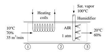
Noting that Q = W = 0, the energy balance on the humidifying section can be expressed as
