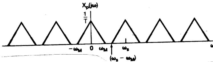
→ Then we can recover  $x(t)$  from  $x_p(t)$  using a low-pass filter.
