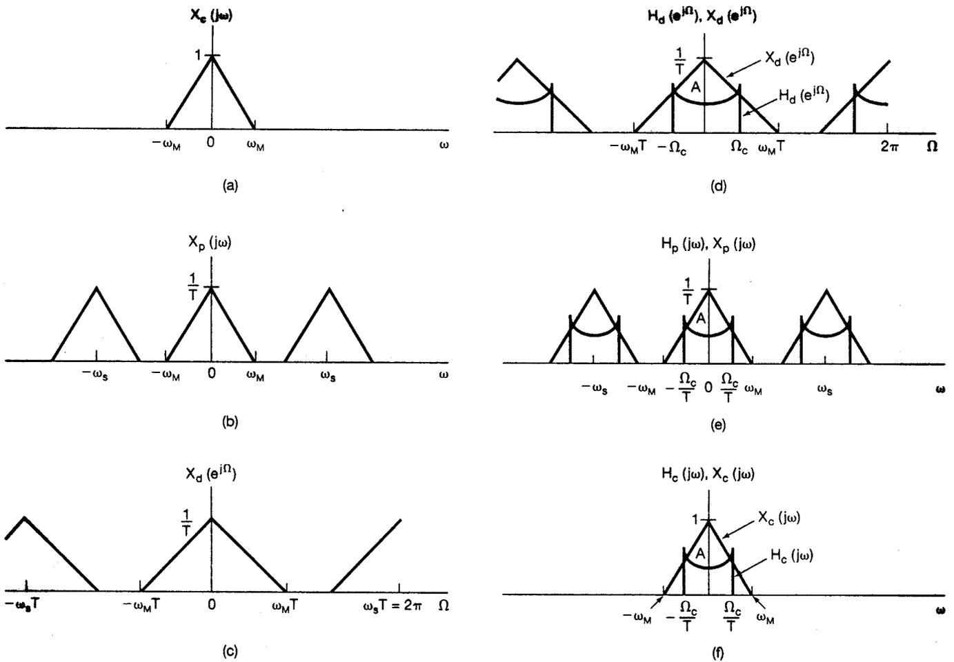
**Figure 7.25** Frequency-domain illustration of the system of Figure 7.24: (a) continuous-time spectrum  $X_c(j\omega)$ ; (b) spectrum after impulse-train sampling; (c) spectrum of discrete-time sequence  $X_d(e^{j\Omega})$ ; (d)  $H_d(e^{j\Omega})$  and  $X_d(e^{j\Omega})$  that are multiplied to form  $Y_d(e^{j\Omega})$ ; (e) spectra that are multiplied to form  $Y_p(j\omega)$ ; (f) spectra that are multiplied to form  $Y_c(j\omega)$ .
