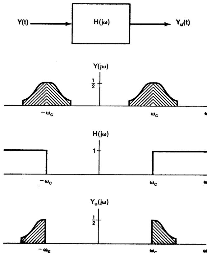
NOTE: The filter must have a very sharp cutoff frequency.
