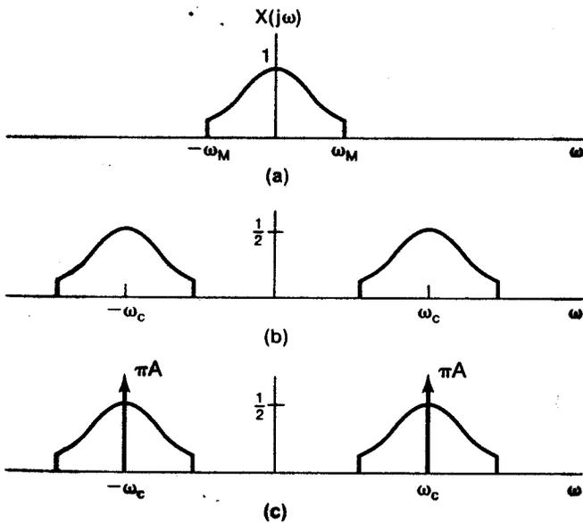
$Y(\omega)$  for synchronous demodulation
