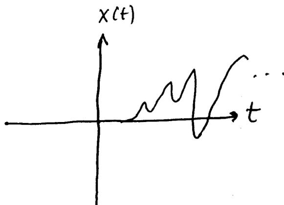
$\Rightarrow$  If  $x(t)$  is right sided and the line  $\text{Re}[s] = \sigma_0$  is in the ROC of  $X(s)$ , then all  $s$  with  $\text{Re}[s] > \sigma_0$  are also in the ROC.
