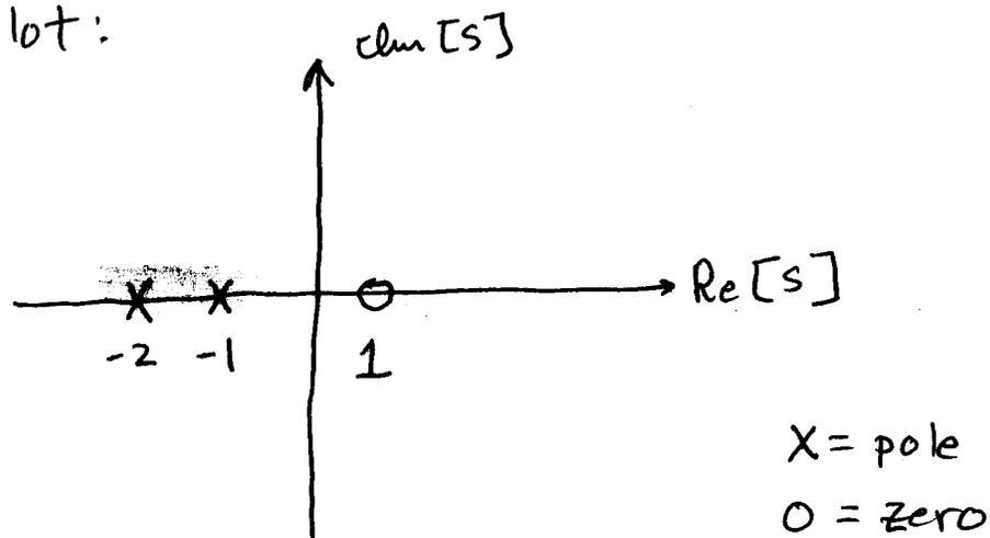
→ Only the finite poles and zeros are shown in the pole-zero plot.
