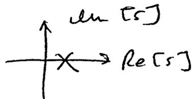
$\Rightarrow$  The system is NOT BIBO stable because  $H(s)$  has a right half-plane pole.
