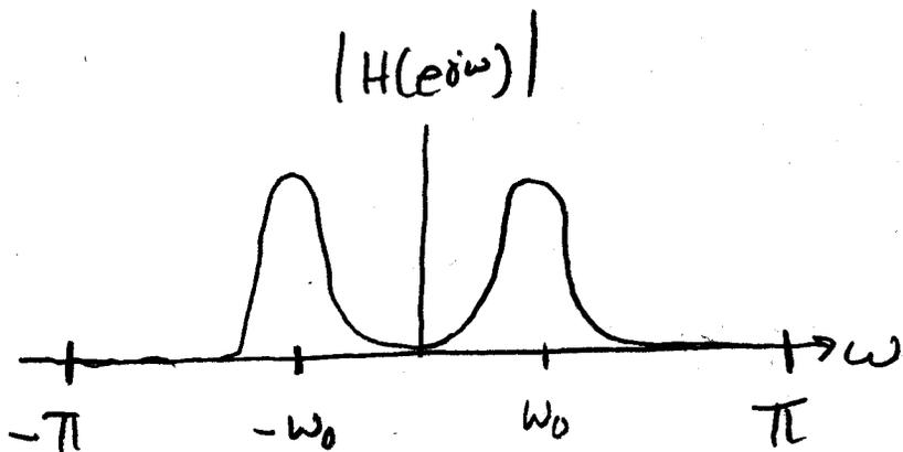
→ So feedback can also be used to alter the frequency characteristic by moving the poles.
